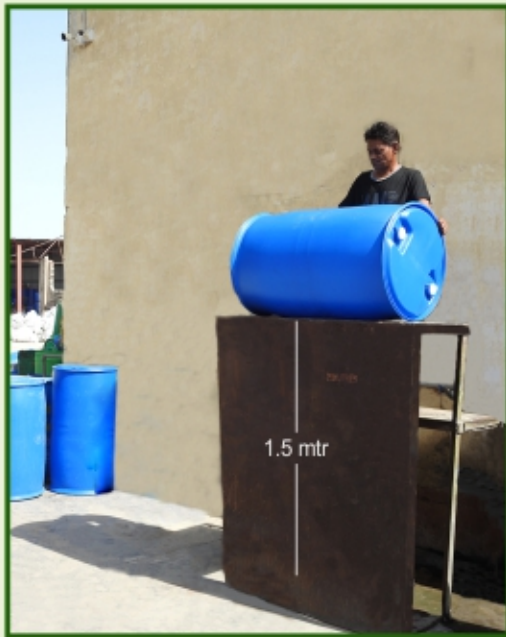
Leakage & Drop Test
