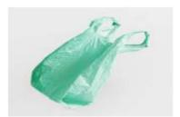
• Low-Density Polyethylene (LDPE): Unlike HDPE, LDPE is characterized by low-density molecules, giving this resin a thinner and more flexible design. It has the simplest structure of all plastics, making it easy and cheap to produce. Used in plastic bags, six-pack rings, various containers, dispensing bottles, and most famously for plastic wraps, it is not often recycled through curbside programs.
